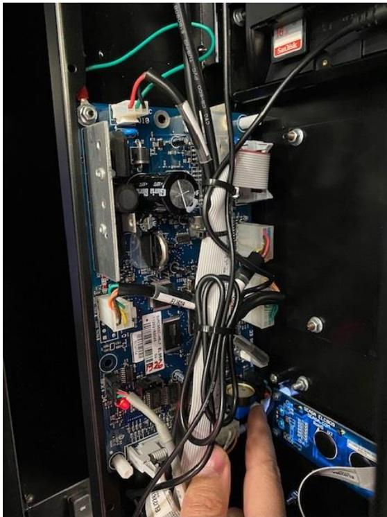
Open the door of the vending machine and press the service menu button (blue) on the VMC (control board) found inside the door.
